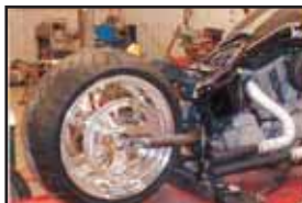
7. Note that if You Swap Fender Struts From Side to Side, You Can Weld Them to Both Sides at the Same Angle. You can re-use these later.
