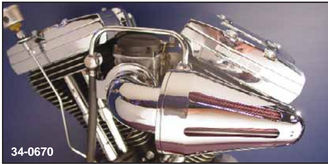
34-0670 installed with 34-0693 adapter
