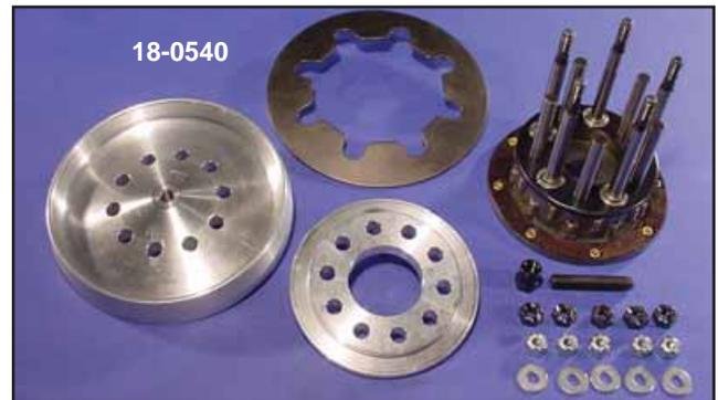
**Sifton Diaphragm Clutch Spring Pressure Plate** for 1941-84 Big Twins. Includes 5-stud clutch, diaphragm spring, pressure plate, rollers, adjustment screw and stud nuts. Use on all Big Twins 1941-64 with open primary and 1965-84 Big Twins with open or closed primary. Updates old style coil spring clutch to new style diaphragm clutch for positive clutch engagement.
